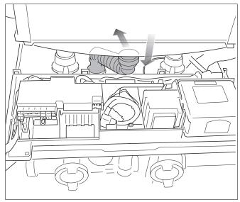
Fig. 91 Removing the condensate trap hose
