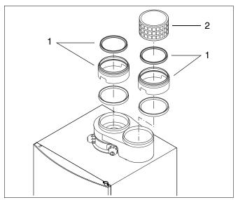
Fig. 19 Connecting the flue gas adapter (parallel)
