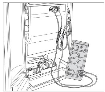
Fig. 68 Measuring the ionization current
