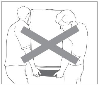
Fig. 6 Incorrect way of lifting and carrying the boiler
