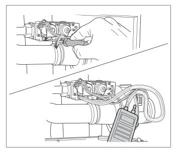
Fig. 77 Checking the gas fitting for internal tightness
