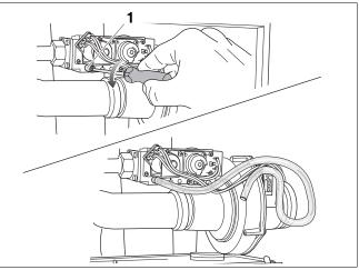
Fig. 53 Bleeding the gas flow pipe
