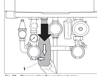
Fig. 90 Disconnecting the condensate trap
