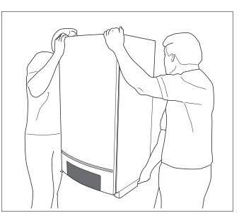
Fig. 5 Lift and carry the boiler correctly
