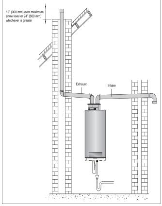
Fig. 26 Vertical venting system (sealed combustion)
