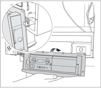
Fig. 98 Hanging the control panel from the boiler frame
