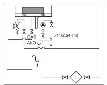
Fig. 16 Connecting the condensate trap
