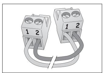
Fig. 40 EMS bus polarity
