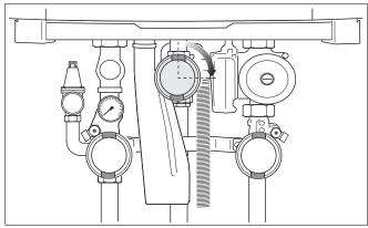
Fig. 73 Closing the gas valve
