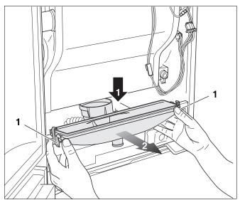
Fig. 92 Removing the condensate collector
