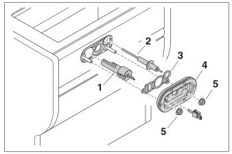
Fig. 88 Replacing the glow ignitor / ionization electrode
