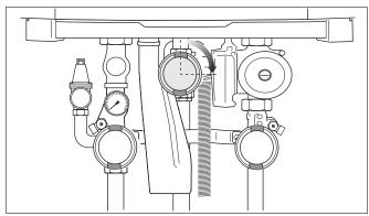
Fig. 52 Closing the gas valve
