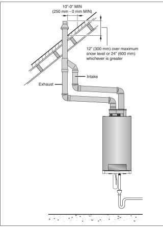
Fig. 28 Vertical venting system (sealed combustion)
