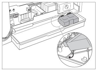
Fig. 36 Clicking the function module into position
