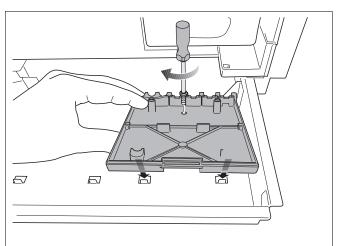
Fig. 35 Installing the wall bracket
