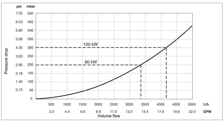
Fig. 99 Boiler resistance curve
