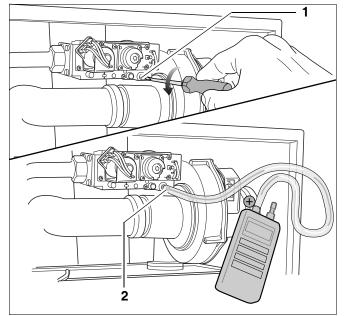
Fig. 60 Checking the gas/air ratio
