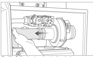
Fig. 82 Pulling the air suction tube from the fan
