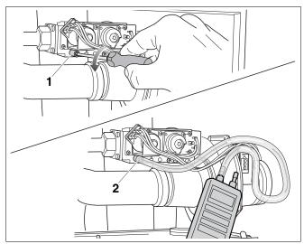
Fig. 57 Measuring the gas supply pressure
