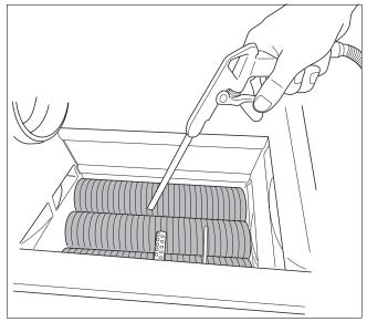
Fig. 94 Cleaning the heat exchanger
