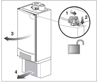
Fig. 47 Opening the boiler door
