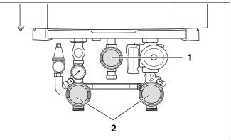
Fig. 78 Closing the valves (here: in closed position)
