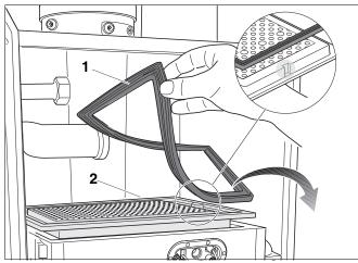
Fig. 85 Removing the burner plate and the burner seal
