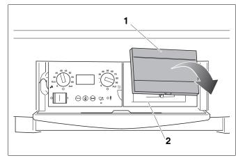
Fig. 33 Remove the cover and install the room controller in the boiler (only for outdoor temperature-dependant operation).
