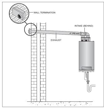
Fig. 27 Horizontal venting system (sealed combustion) -Situation 2 (PVC only)
