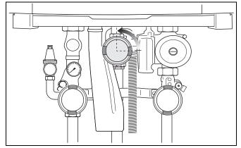
Fig. 54 Opening the gas valve
