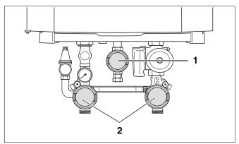
Fig. 75 Closing the valves (here: in closed position)
