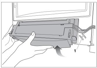
Fig. 97 Removing the control panel
