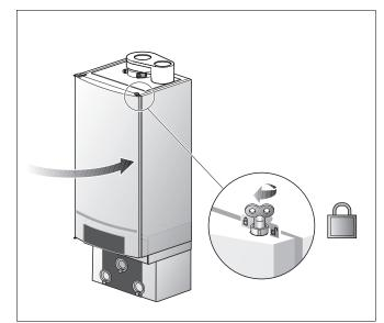
Fig. 71 Closing the boiler door
