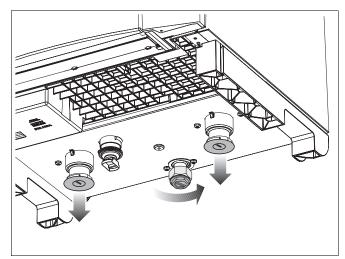
Fig. 9 Removing the covers – boiler bottom
