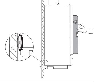
Fig. 8 Aligning the boiler with the set screw
