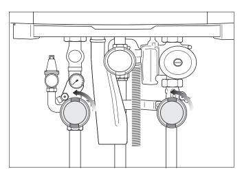
Fig. 49 Opening the isolating valves (here: open position)
