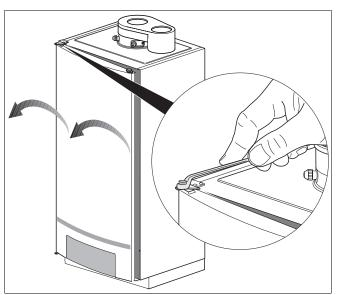
Fig. 79 Removing the boiler door
