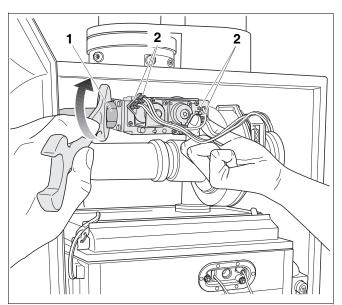
Fig. 80 Undoing the connections to the gas fitting
