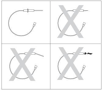
Fig. 87 Checking the ionization electrode
