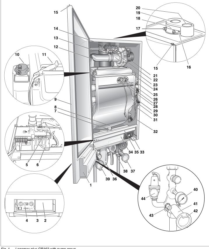
Fig. 1 Logamax plus GB162 with pump group
