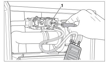
Fig. 62 Adjusting the gas/air ratio
