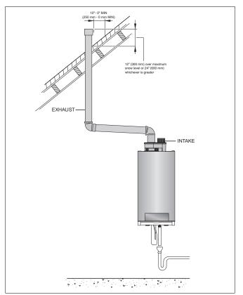
Fig. 23 Vertical venting system (room air only)
