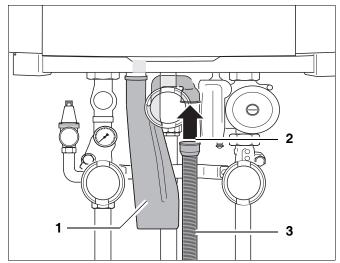
Fig. 15 Installing the condensate trap hose
