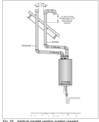
Fig. 25 Vertical parallel venting system (sealed combustion) - Situation 1
