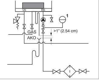
Fig. 18 Connecting the expansion vessel in a single-boiler system
