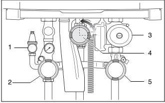
Fig. 45 Open the gas valve
