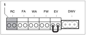
Fig. 41 External connection board - Room controller RC and EMS bus (connection color orange)
