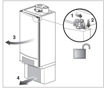
Fig. 76 Opening the boiler door
