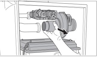
Fig. 84 Removing the burner cover with the gas/air unit
