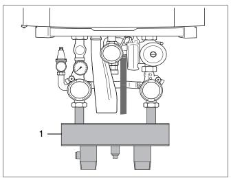
Fig. 11 Low loss header
