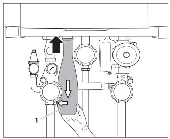
Fig. 14 Installing the condensate trap
