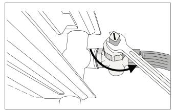
Fig. 74 Draining the heating system (example)
