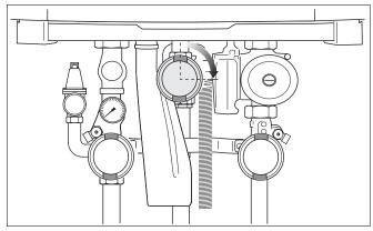
Fig. 56 Closing the gas valve
