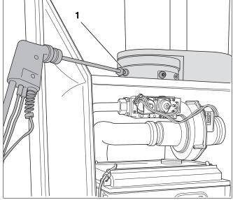
Fig. 65 Measuring the gas supply pressure
