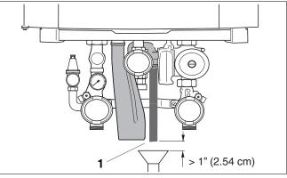
Fig. 17 Condensate drainage pipe
