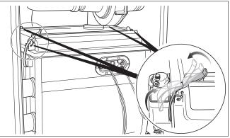
Fig. 83 Opening the retaining clips
