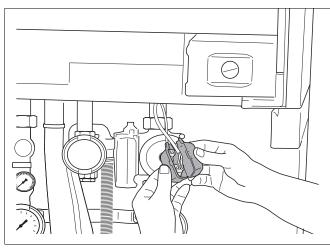
Fig. 37 Removing the covers
