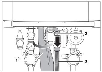
Fig. 89 Disconnecting the condensate trap hose
