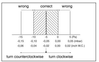
Fig. 61 Air/gas difference at part load
