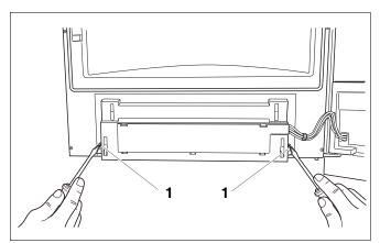
Fig. 96 Loosening the screws
