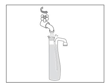
Fig. 51 Filling the condensate trap with water
