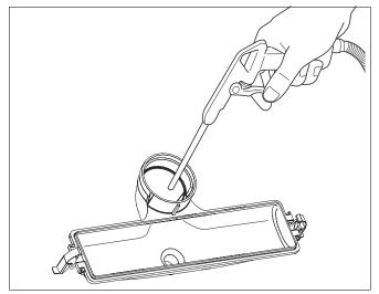
Fig. 93 Cleaning the condensate collector
