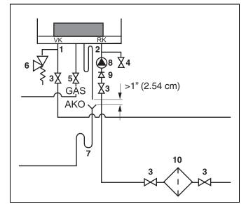
Fig. 12 Connecting the boiler supply and return
