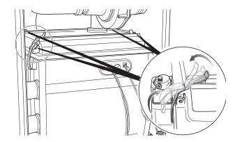
• Open the 4 snap closures of the burner cover.
