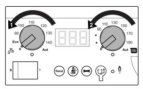
Put the selector for the DHW temperature setting [1] and the selector for the maximum heating-system supply temperature [2] in position "0".
