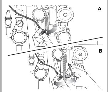
Undo the pump power supply cord plug as instructed in A, [1] and B, [1].
