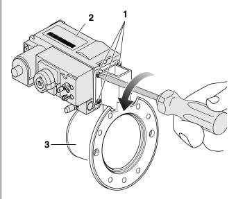
100 kW: Loosen the 4 torx screws [1] and remove the gas valve [2] from the venturi pipe [3].
