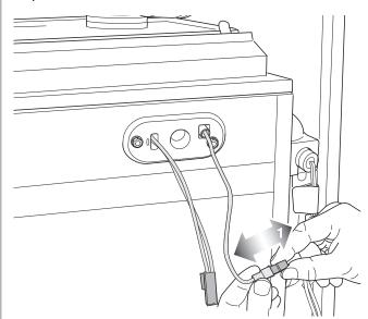
Disconnect the plug of the ionization electrode [1].
