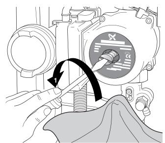
Drain the pump by removing the vent screw at the front of the pump [1].
