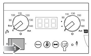
Put the main power switch [1] on the control panel in position "1" (On).
