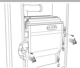
Loosen both mounting screws [1].
