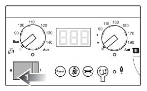
Put the main power switch [1] on the control panel in position "0" (Off).
