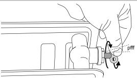
Purge all radiators in the heating system. Start at the lowest floor of the premises and then work your way up from floor to floor.
