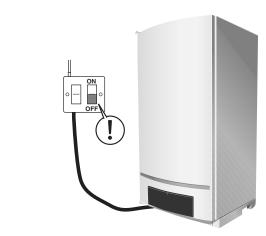
• Switch off the power supply to the heating system.
