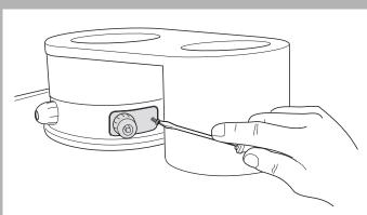
Remove the cap from the measuring nipple of the combustion air supply.
