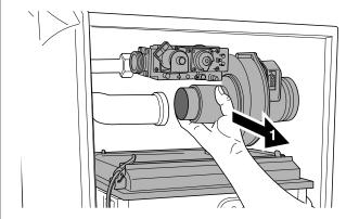
Remove the gas/air unit including the burner cover [1] by moving it in the direction indicated by the arrow.
