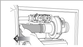
• Pull the air suction pipe from the venturi pipe [3].
