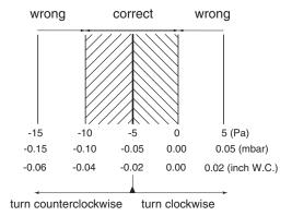
Check the gas/air ratio. The gas/air ratio is measured as a pressure difference between the pressure in the gas valve and the ambient pressure. This pressure difference must be between -0.04 – 0 inch W.C. As a result, the nominal pressure difference is -0.02 inch W.C.
