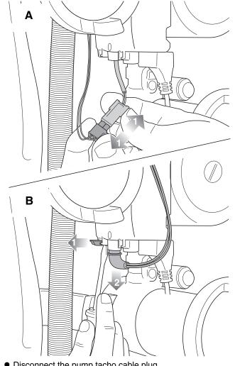
Disconnect the pump tacho cable plug.
