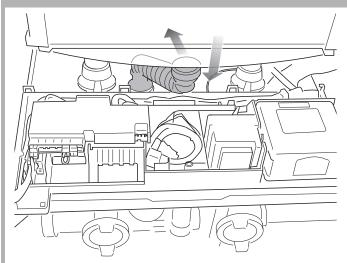
Pull the condensate draining pipe down and bend it backwards.
