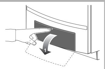
• Open the cover of the BC10 on the front of the boiler [1].
