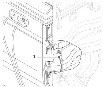
• Check that the ground lead of the ionization circuit [1] has been installed correctly.
