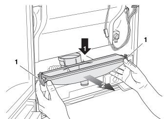
Open the 2 snap closures [1] on the left and the right and remove the condensate water tank.
