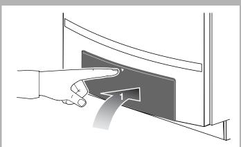
• Close the cover of the BC10 on the front of the boiler [1].
