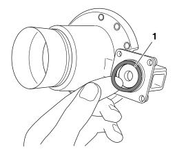
• Install a new O-ring [1] in the venturi pipe.
