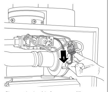
Disconnect the plug of the flue gas sensor [1].
