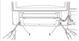
• Loosen the 2 screws on the back of the door of the BC10 [1].
