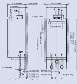
The required permanent clearances (closet) are: front: 1" (25 mm) right side: 0 left side: 0 above: 6" (152 mm) The position selected for installation MUST allow adequate space for servicing in front of the boiler of at
