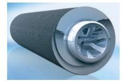
on the outside of the aluminum tube increase the exterior surface area. This means more hot flue gas comes into contact with the heat exchanger to maximize heat transfer. A spiral channel on the inside of the tube increases the internal surface area and creates turbulence, bringing more water into contact with the heating surface, also
