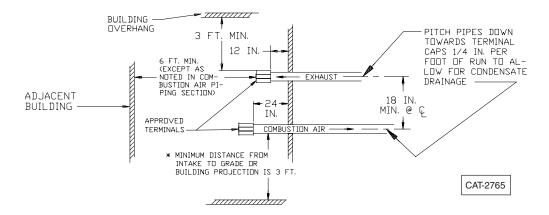
Figure 10. Vertical Vent Installation
