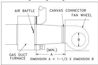
Figure 3 - Recommended Ductwork Design for Elbowed Arrangement
