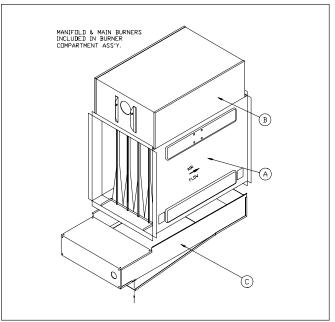
Figure 16 - Power Venter Assembly
