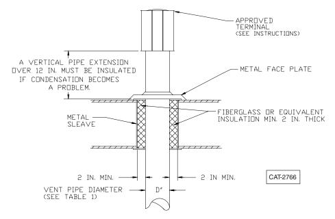
Figure 10A. Horizontal Vent Installation
