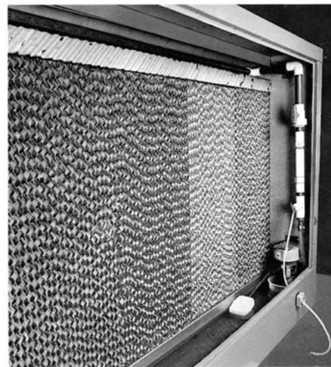
Internal View Evaporative Cooler
