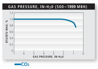
The Futera III provides high tolerance for real world conditions as it maintains 100% full input down to 2"wc.
