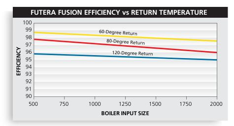
Unlike most condensing products available today which publish highest efficiencies at lowest inputs, the Futera Fusion is capable of attaining efficiencies as high as 98% at full input.
