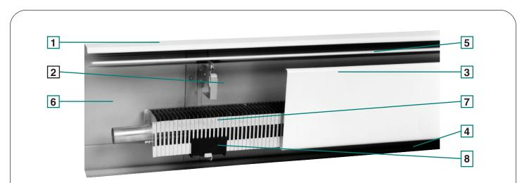
I - ENCLOSURE TOP AND BACK PANEL - is of one-piece steel construction for strength and durability. Smooth surface won't collect dust and lint. Lower portion is extended 3/4" out from wall to cover any openings between wall and finished flooring and to let panel stand unaided while being fastened to wall.
