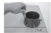
Secure vent collar with 4 screws to the top panel.
