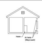
Eternal takes combustion air from surrounding. It does not take combustion air directly from outside. Therefore, make sure the area has access to fresh air. If installing in closet make sure louvers are installed to provide air. Check your install space to see if air is supplied from within your home or from outside.
