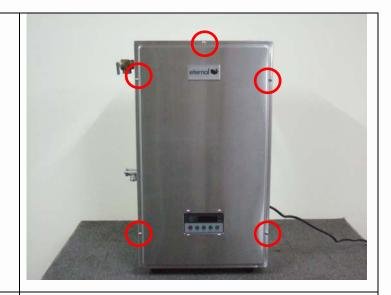
Loosen the screw to open the PCB Main Controller Cover
