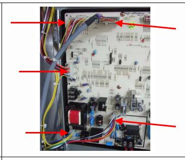
Remove the two Philips head screws to loosen the power supply wiring
