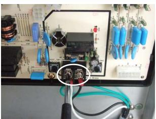
Remove the four Philips head screws and PCB Main Controller Board comes right out
