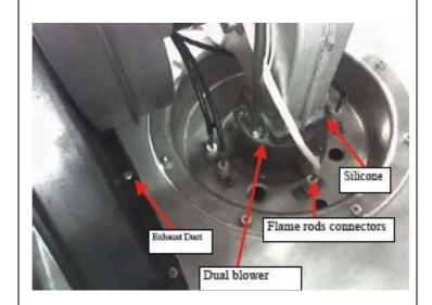
Gently remove the dual blower assembly; the injection blower is secured by silicone sealant so some force may be required
