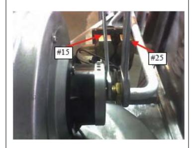
Loosen two screws to remove the heat exchanger thermostat switch
