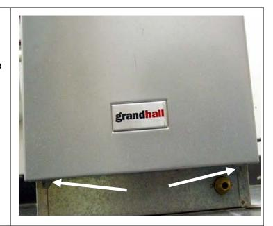
Remove the three Phillips head screws attaching the vinyl cover.
