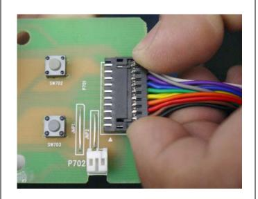
Once the Wire Connector is free reverse these steps to reinstall new LED Display.
