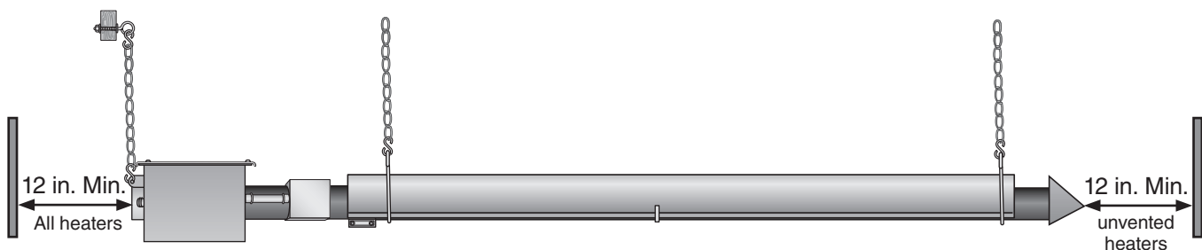
Figure 3.25 • Minimum End Clearances
