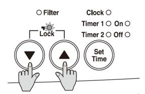
To deactivate Function Lock simply press the " $\blacktriangle$ " and " $\checkmark$ " buttons at the same time for 2 seconds and the Function Lock indicator will go out.
