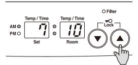
3. Press the Set Time button again, the Timer 1 OFF indicator will glow. Press the "▲" button until AM 9:00 appears.
