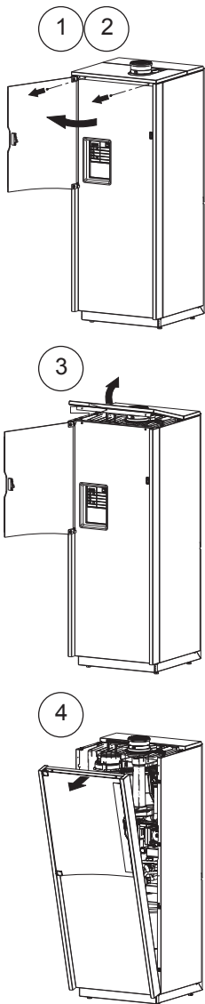
Removing casing parts Q Premier
