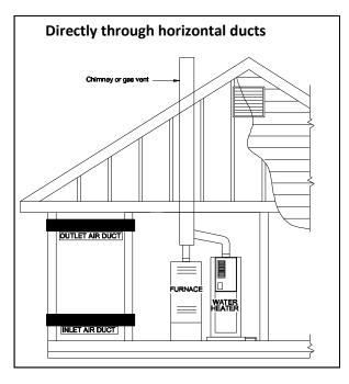
When communicating directly with the outdoors through horizontal ducts, each opening shall have a minimum free area of 1 in<sup>2</sup>/2000 Btu/hr (1100 mm<sup>2</sup>/kW) of total input rating of all appliances in the confined space.
