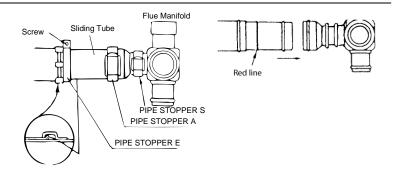
Slide the insulation sleeve up to the flue manifold and slip the securing clip over the sleeve as shown.
