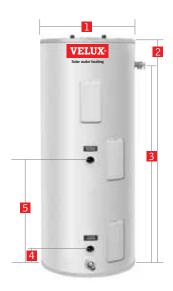
Solar storage tank with electric backup • Glass lined steel tank • Two protective aluminum anode rods • 2" non-CFC foam insulation (R-17) • Double wall solar heat exchanger • Sensor wires for solar thermistor connections • Dual backup heating elements • <sup>3</sup>/<sub>4</sub>" solar supply and return connections • <sup>3</sup>/<sub>4</sub>" potable water connections • Direct heat transfer with immersed incoloy elements • T & P relief valve Brass drain valve
