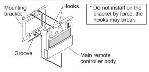
6. Secure the remote using the machine screws.
