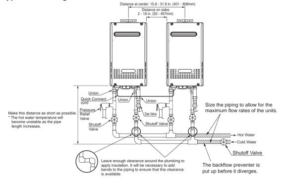
Insulate the hot water piping to prevent heat loss. Insulate and apply heating materials to the cold water supply piping to prevent heat loss and freezing of pipes when exposed to excessively cold temperatures.
