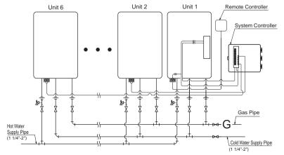
• Insulate or apply heating materials to both the cold water supply piping and the hot water supply piping to prevent freezing during cold weather and to prevent heat loss through the piping.
