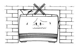
The flue is not designed to be positioned under floors, or below the level of the heater.
