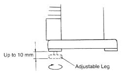
If necessary, the unit can be leveled using the adjustable legs under the front right and left hand side legs.
