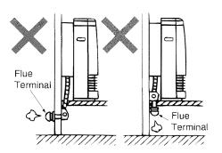
The flue terminal should be positioned away from flammable materials.
