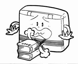
Do not spray aerosols while the heater is operating. Most aerosols contain butane gas, and can be a fire hazard if used near this heater when it is in use.
