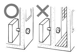
Flue may be positioned directly under opening windows, with a minimum clearance of 9" (230mm).
