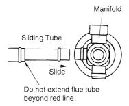
2. Fit the locking clamp over connection between sliding tube and manifold. Engage the hook and rotate it until it snaps against the body of the clamp.
