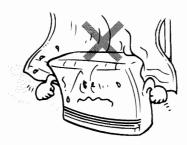
Combustible materials must not be placed where the heater could ignite them.
