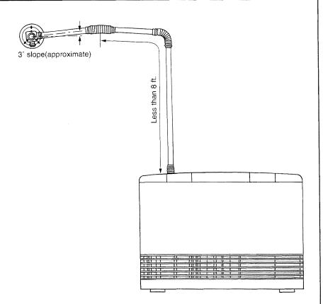
4. Wherever the air intake hose and exhaust pipe run sideways, try to have the exhaust pipe on top (to prevent the air intake hose from sagging onto the exhaust pipe).
