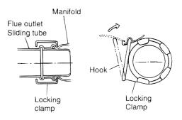
3. Fit the screw clamp between the sliding tube and the flue elbow. Secure with the 4mm screws supplied. The flue outlet is now locked into position.
