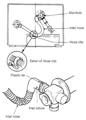
When servicing unit replace plastic tie with new one. (Available at local hardware store or contact local distributor.)
