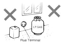
Do not flue into natural draught flues or fireplaces, this unit can only be used with one of the five types of Rinnai flue kits. Do not flue unit into other rooms. Flue terminal must be outside.
