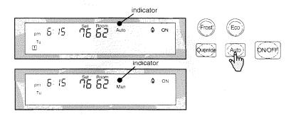
3 Select the desired room temperature by pressing the "▲" or "▼" buttons.
