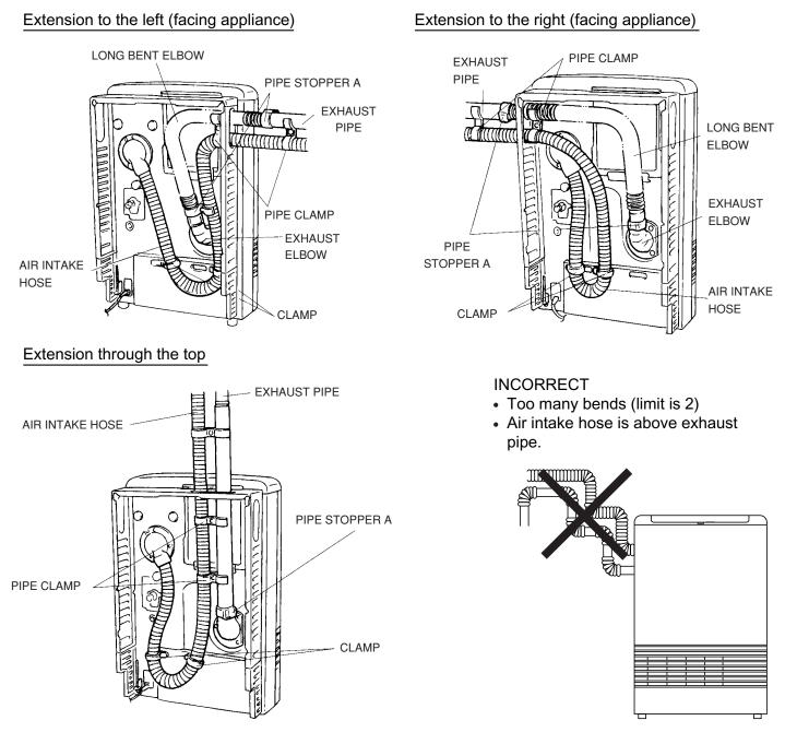
**CAUTION** Use the pipe stoppers, connectors, clamps, and screws according to these instructions in order to ensure no leakage of exhaust gases.
