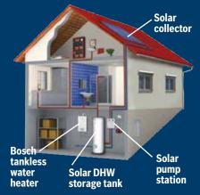
The sunlight heats up a fluid inside the collector. This fluid transfers the heat to the DHW tank. Right away you profit from solar energy, either when you shower, do laundry, wash dishes, and all other hot water needs.
