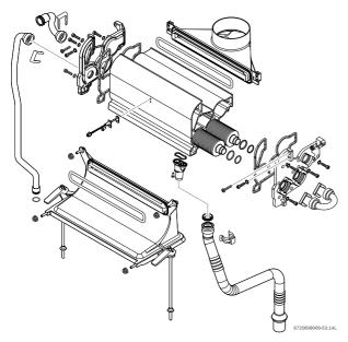
Fig. 60 Condensing heat exchanger
