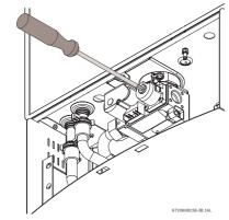
Fig. 64 Adjusting P2 CO<sub>2</sub> level
