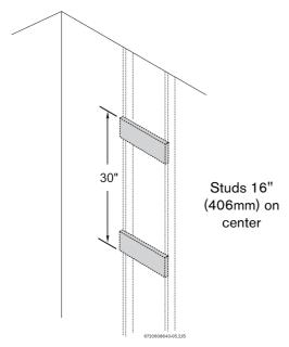
Fig. 8 Distance between support boards
