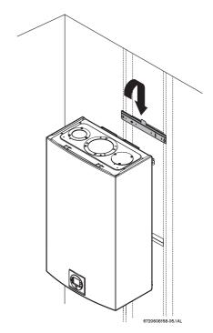
Fig. 10 Mounting the heater
