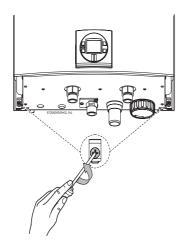
Fig. 3 Loosen the two screws
