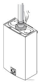
Fig. 23 Exhaust connection
