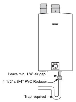
Fig. 34 Appliance drain installation
