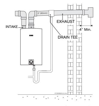
Fig. 32 Horizontal venting system (room air only)
