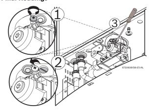
Fig. 63 Adjusting P1 CO<sub>2</sub> level
