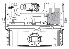
Fig. 22 Water level in condensate trap
