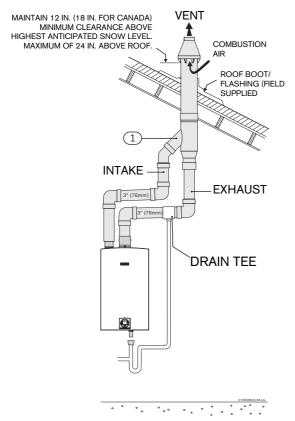
Fig. 26 Vertical venting system (sealed combustion)
