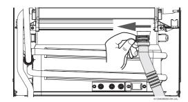
Fig. 19 Disconnect drain tube
