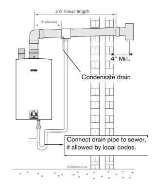
Fig. 35 External condensate drain installation
