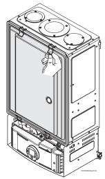
Fig. 5 Remove the combustion cover
