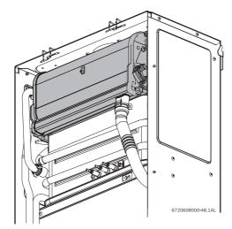
Fig. 59 Condensing heat exchanger unit
