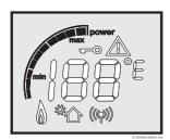
Fig. 42 Power bar indicator (input)
