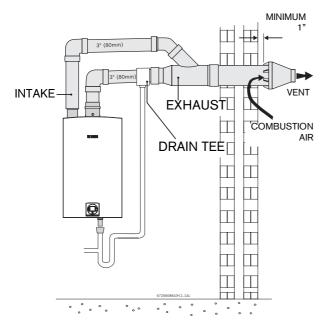
Fig. 29 Horizontal venting system (sealed combustion)
