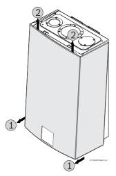
Fig. 4 Remove the front cover
