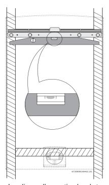
Fig. 9 Leveling wall mounting bracket
