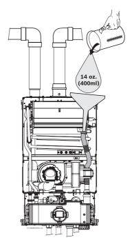
Fig. 20 Filling the condensate trap after installation
