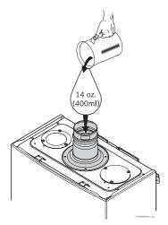
Fig. 18 Filling the condensate trap at start up
