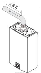
The minimum exhaust vent length is 3 feet (1 m) with one 90 degree elbow.
