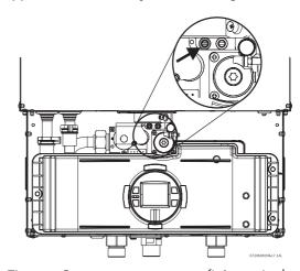
Fig. 38 Gas pressure test port (left tapping)
