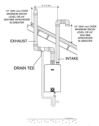
Fig. 27 Vertical parallel venting system (sealed combustion)
