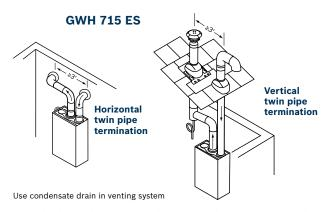
NOTE: The distance between the combustion air intake pipe termination and the exhaust pipe termination must be greater than or equal to 3 feet.
