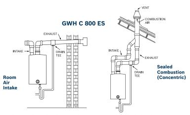
Ships complete with wall mounting bracket, pressure relief valve, built-in electronic temperature controls and 120V plug-in power cord. Refer to manual for condensate drain tee and venting requirements.
