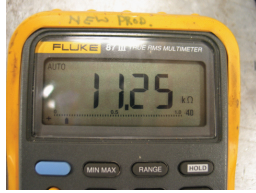
Fig. 20 – Measuring Scroll NTC Resistance
