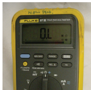
Fig. 22 – Checking NTC Circuit for Grounded Condition
