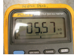
Fig. 21 – Measuring Motor NTC Resistance
