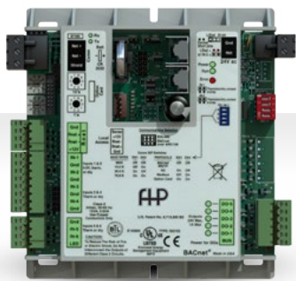
DDC Control Board
