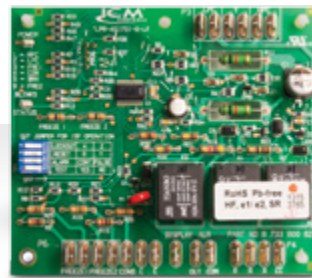
UPM Control Board
