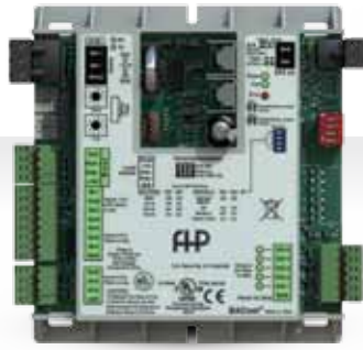
DDC Control Board
