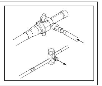
**STEP 4** - Wrap a wet rag around the valve body to avoid heat damage and continue the dry nitrogen purge.
