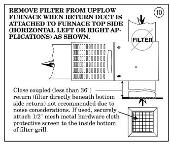
If only the front of the furnace is accessible, it is recommended that both supply and return air plenums are removable.
