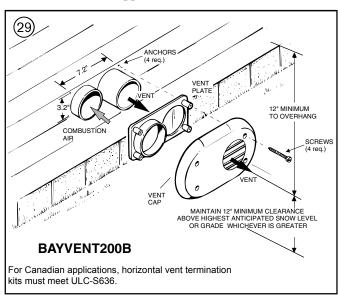
**PITCH** – Venting through the wall must maintain 1/4" per foot pitched upward to insure that condensate drains back to the furnace.
