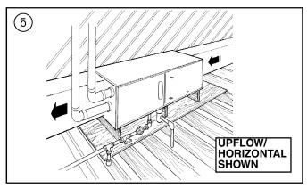
The furnace must be supported at both ends and the middle when installed horizontally.
