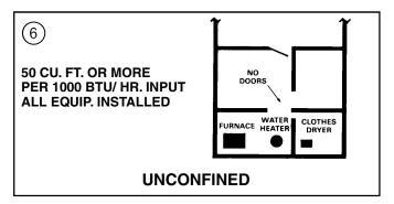
Provisions for combustion and ventilation air shall be made in accordance with latest edition of Section 5.3, Air for Combustion and Ventilation, of the National Fuel Gas Code, ANSI Z223.1 — CAN/ CGA B149.1 or applicable provisions of the local building codes. Special conditions created by mechanical exhausting of air and fireplaces must be considered to avoid unsatisfactory furnace operation.
