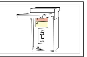
**STEP 4** - Wait one (1) hour before starting the unit if compressor crankcase heater accessory is used and the Outdoor Ambient is below 70°F.
