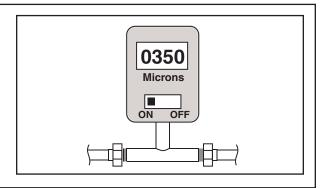
**STEP 2** - Observe the micron gauge. Evacuation is complete if the micron gauge does not rise above 500 microns in one (1) minute.
