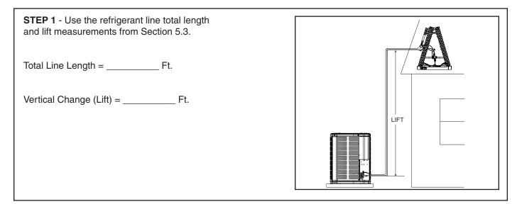
STEP 2 - Determine the final subcooling value using total Line Length and Lift measured in STEP 1 and the charts below.
