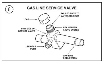
6. Precautions should be taken to avoid heat damage to the pressure tap valve core during brazing. It is recommended that the pressure tap port valve core be removed and a wet rag wrapped around the valve body.
