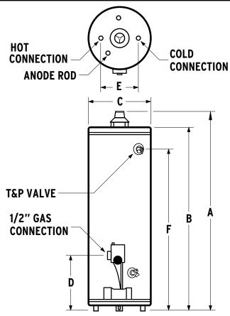
Maximum Hydrostatic Working Pressure: 150 PSI.
