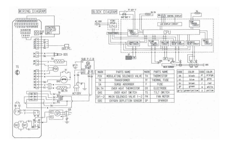
If any of the original wire as supplied with the appliance must be replaced, it must be replaced with a wire of a least a 194°F temperature rating and number 18AWG or its equivalent. "CAUTION: Label all wires prior to disconnection when servicing controls. Wiring errors can cause improper and dangerous operation." Verify operation after servicing.
