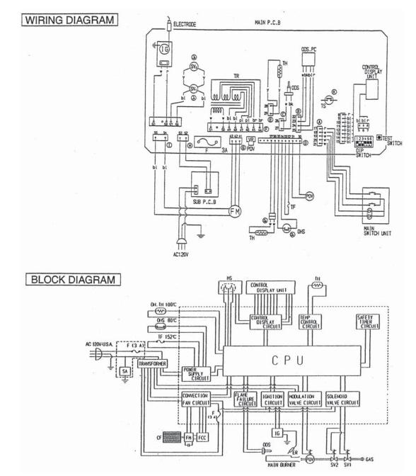
If any of the original wire as supplied with the appliance must be replaced, it must be replaced with a wire of a least a 194°F temperature rating and number 18AWG or its equivalent. "CAUTION: Label all wires prior to disconnection when servicing controls. Wiring errors can cause improper and dangerous operation." Verify operation after servicing.
