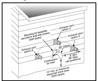
Figure 7. Inlet & Exhaust Pipe Clearances
