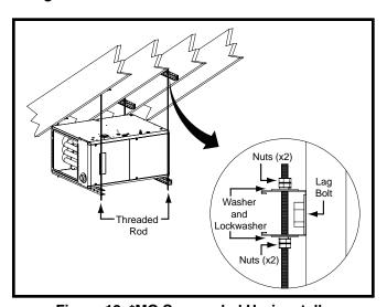
Figure 12. \*MQ Suspended Horizontally
