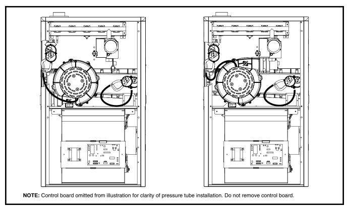
Figure 17. Pressure Switch Tubing for \*MQ Upflow / Horizontal Furnaces
