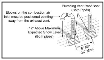
**Figure 10. Vertical Vent Termination**
