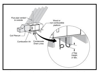
Figure 11. Horizontal installation on a Platform
