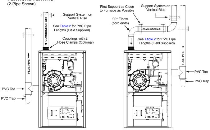
Figure 28. Horizontal & Vertical Venting Options
