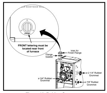
Figure 15. Rubber Grommets
