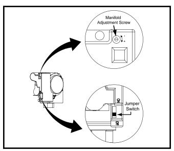
Figure 21. Modulating Gas Valve
