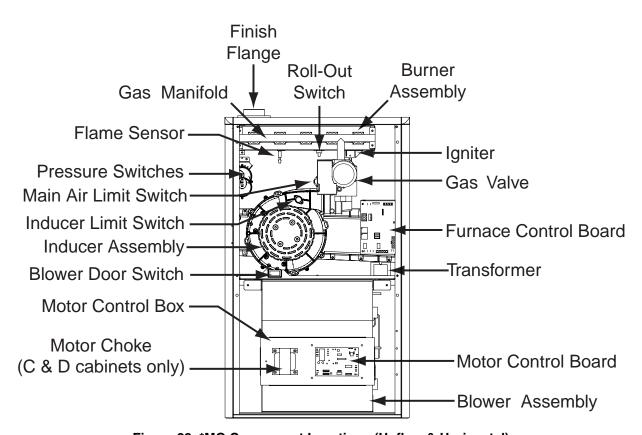
Figure 29. \*MQ Component Locations (Upflow & Horizontal)
