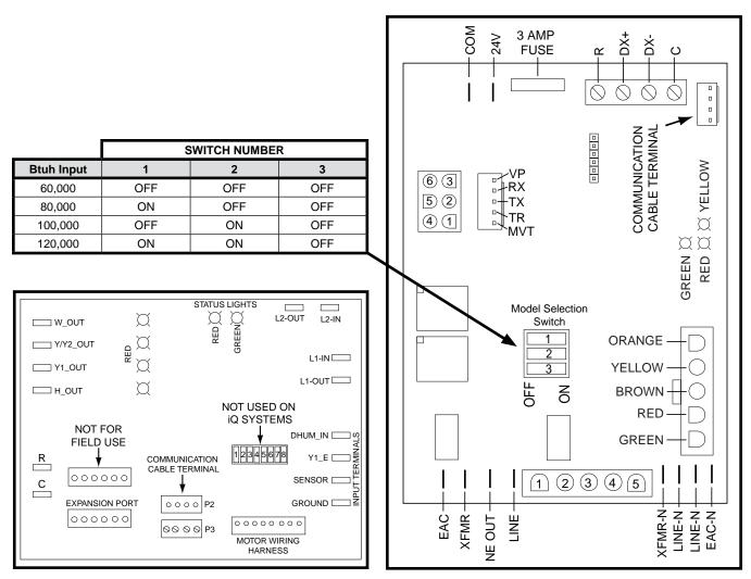
Figure 23. Variable Speed Motor Control Board
