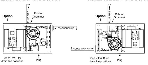
Figure 27. Vent Pipe & Condensate Options - Horizontal Furnaces
