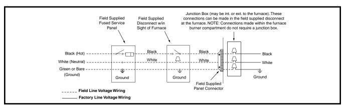
Figure 19. Line Voltage Field Wiring
