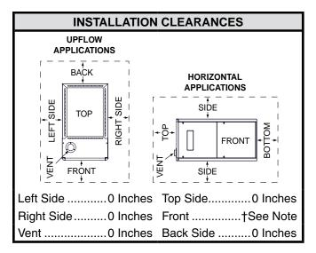
**NOTE:** Allow 24 inches minimum clearance for servicing. Recommended clearance is 36 inches.
