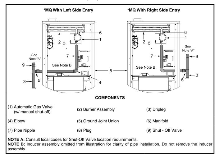
Figure 18. Typical Gas Connections
