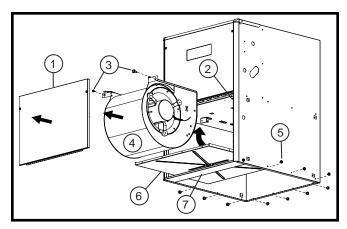
Figure 13. Bottom Panel Removal
