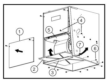
Figure 14. Alternate Removal Method
