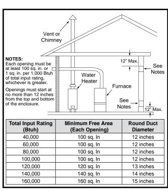
Figure 2. Combustion Air Drawn from Inside
