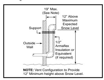
Figure 9. Alternate Horizontal Vent Installation
