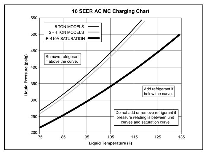
Figure 5. Charging Chart for 2-5 Ton Units
