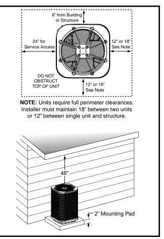
Figure 1. Clearance Requirements
