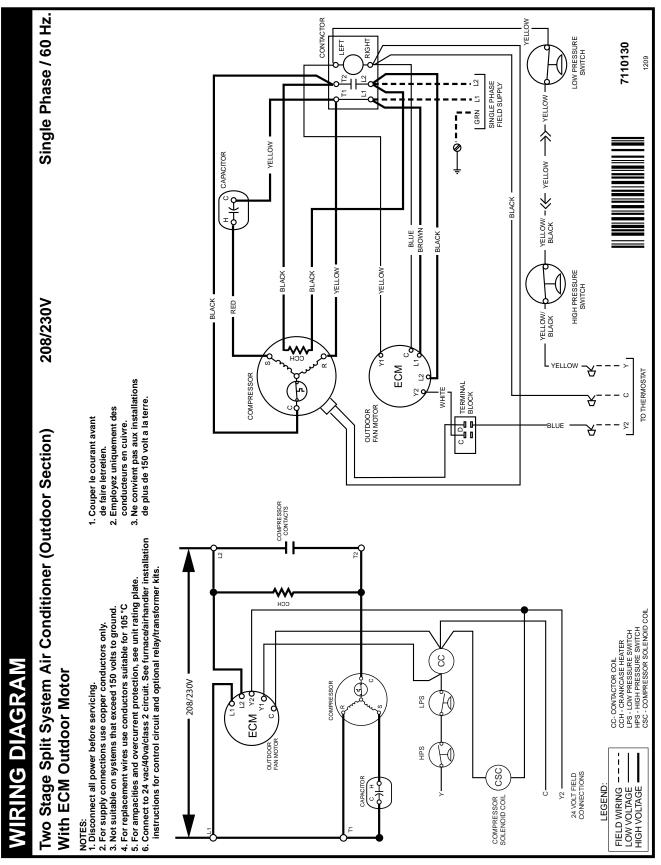
Figure 10. Wiring Diagram for S4BF-048 & S4BF-060 (4 & 5 Ton) Series
