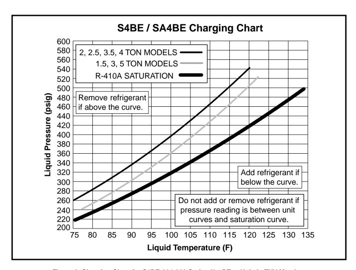
Figure 3. Charging Chart for S4BE-024-060 Series (2 - 5 Ton Units) - TXV Matches
