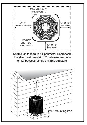
Figure 1. Clearance Requirements
