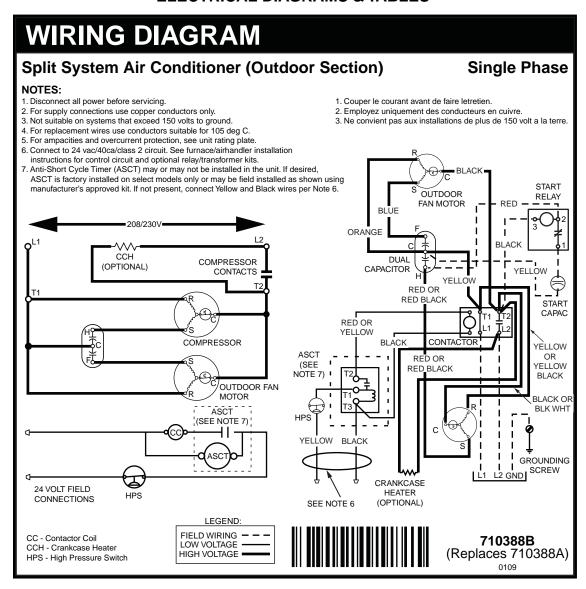
Figure 4. Single Phase Air Conditioner without CoreSense™ (1.5 - 4 Ton Models)
