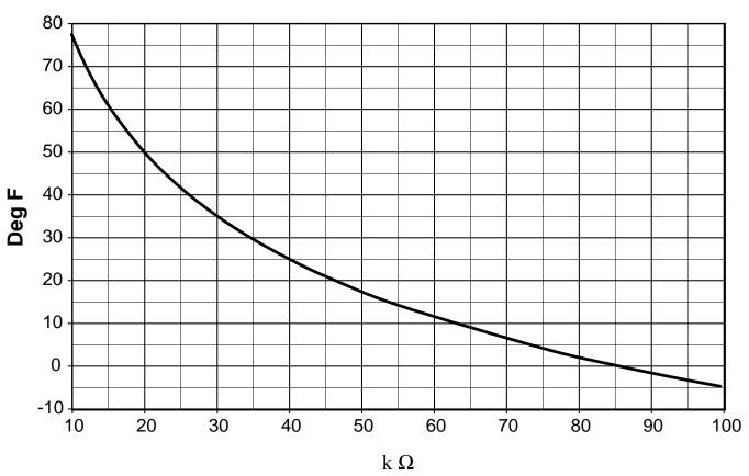
**Figure 10. Temperature Sensor Resistance Charts**
