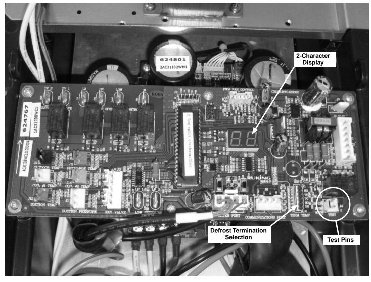
Figure 7. Interface Board in Control Panel
