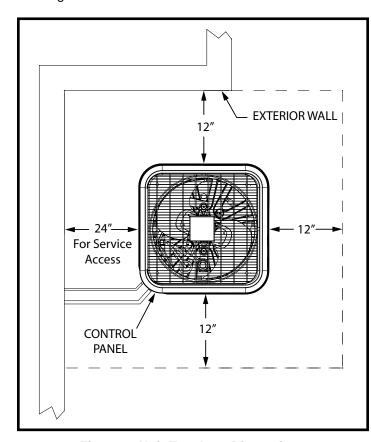
Figure 1. Unit Envelope Dimensions
