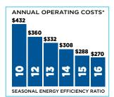
\* Annual costs based on 36,000 Btu unit, 1500 cooling load hours, and .08/kwh. Actual costs may vary depending on climate conditions, energy rates and patterns of usage.
