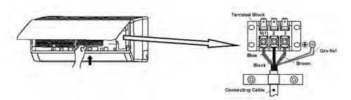
3. Connect wiring to indoor unit per connection diagram.
