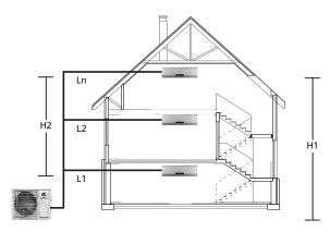
Measure and record the piping length (L1,L2, L3....Ln) from the outdoor unit to each indoor unit.
