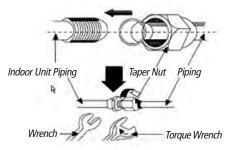
10. Carefully tighten flare nuts to correct torque level referring to the following Torque Table:
