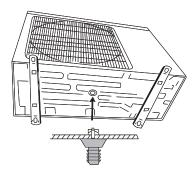
Drain Fitting Installation
