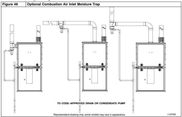
The External Vent Trap Kit accessory may be used as a trap for the combustion air inlet pipe if a large amount of moisture must be removed. The drain line may be connected to the same drain as the furnace condensate and the evaporator coil condensate line ONLY if the inlet air trap drain and the evaporator coil drain empty into an open segment of pipe above the drain, See **Figure 12**. When using the External Vent Trap Kit, refer to those instructions for proper drain connections.
