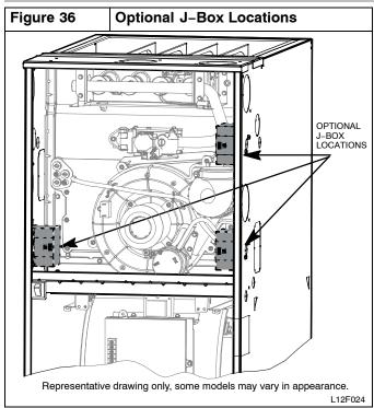
Remove the J-Box cover and mounting bracket from the loose parts bag. Select a 7/8-in. (22 mm) knock-out on the desired side of the casing. Remove the knock-out from the casing. Drill two 1/8-in. (3 mm) pilot holes in the casing dimples by the desired 7/8-in. (22 mm) knock-out.
