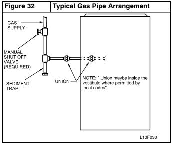
A 1/8-in. (3 mm) NPT plugged tapping, accessible for test gauge connection, MUST be installed immediately upstream of gas supply connection to furnace and downstream of manual equipment shutoff valve.
