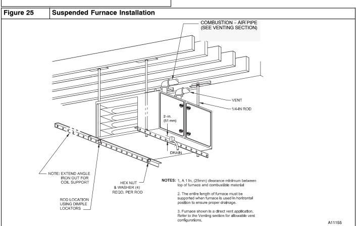
NOTE: Local codes may require a drain pan and condensate trap when a condensing furnace is installed over a finished ceiling
