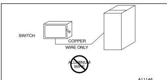
Use a separate, fused branch electrical circuit with a properly sized fuse or circuit breaker for this furnace. See **Table 11** for wire size and fuse specifications. A readily accessible means of electrical disconnect must be located within sight of the furnace.
