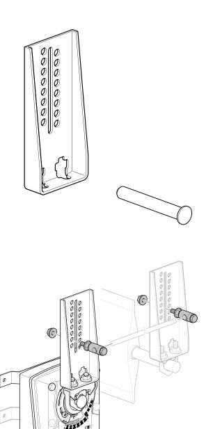
Non-direct mounting with ZG-EFB crank arm adaptor kit
