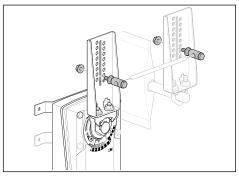
Linkage solutions are available when direct coupling is not possible.
