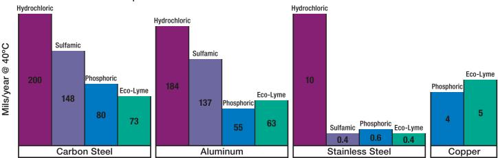
Comparative Corrosion Rates of Common Descaler Chemistries
