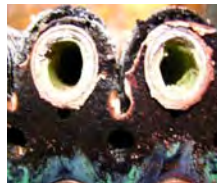
Scale Build up from untreated water.
