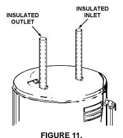
Fit pipe insulation over the incoming cold water line and the hot water line. Make sure that the insulation is against the top cover of the heater. Fit T & P valve insulation over valve. Make sure that the insulation does not interfere with the lever of the T & P valve.
