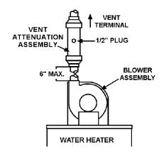
FIGURE 22: Typical Vertical Installation
