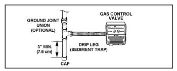
FIGURE 12. GAS PIPING WITH FLEXIBLE CONNECTOR.
