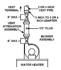
FIGURE 24: Typical Installation for Vertical Vent with 3 or 4 inch Pipe
