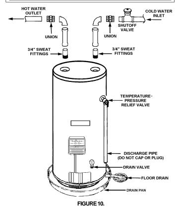
Figure 10 shows the typical attachment of the water piping to the water heater. The water heater is equipped with 3/4 inch NPT water connections.
