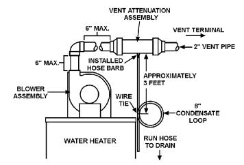
FIGURE 23: Typical Horizontal Installation
