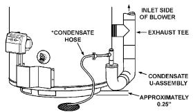
\*NOTE: NO PORTION OF THE CONDENSATE HOSE MAY BE ELEVATED HIGHER THAN THE CLAMP THAT IS SECURED TO THE SIDE OF THE JACKET THROUGHOUT THE ENTIRE LENGTH OF THE HOSE INCLUDING THE EXIT INTO AN APPROPRIATE DRAIN.
