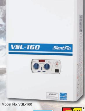
The stainless steel primary exchanger with shared radial circulation, the VSL160 air/gas modulation system, the Acquajet DHW exchanger and the Hydroplus electronic control are all European design and tested. The Slant/Fin VSL-160 condensing gas boiler stands at the top in performance, safety and environmental ratings. The boiler is equipped
