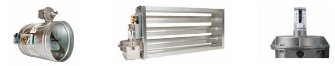
The EBD style by-pass are self-contained units that give you the static control mounted to the damper. It is an "all-inone" design that makes the installation process much easier than most electronic by-pass dampers. The static pressure can be adjusted in the field between 0.1" to 4" of pressure. This is done by the turn of a set-screw. Requires 24VAC to operate. Tubing and pitot tube are included.
